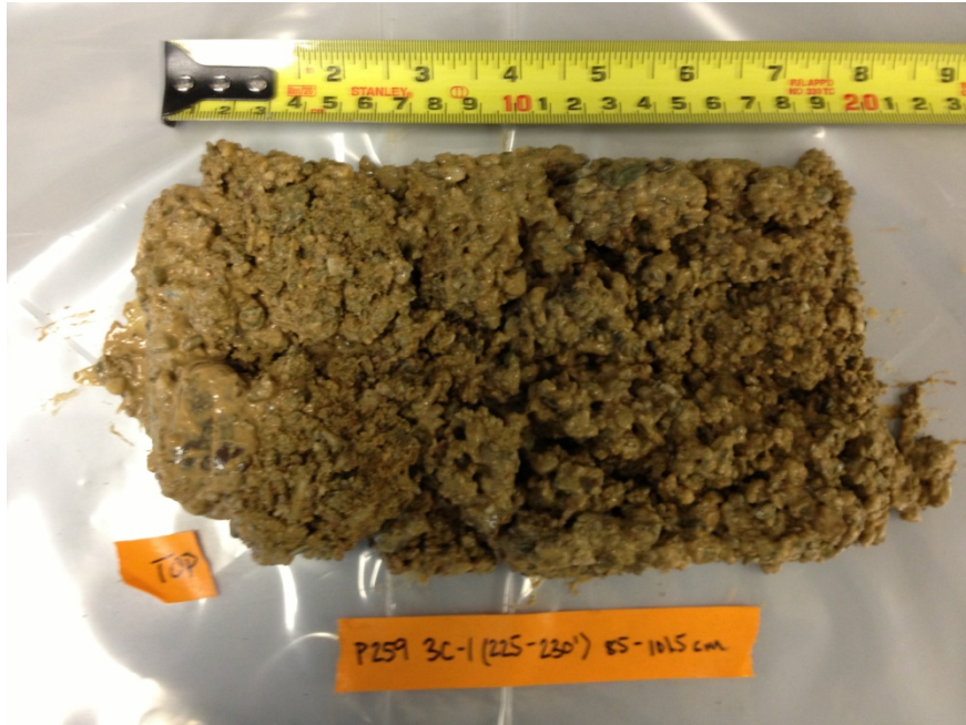
P259-3C (227.8-228.3 ft bgs): muddy gravel w/some sand
